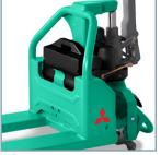
**#2** The PBPL's 48V lithium ion power source charges in just 3.5 hours and offers 6 hours of use.
