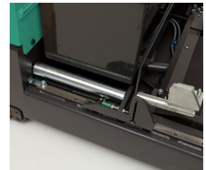
Battery on rollers
