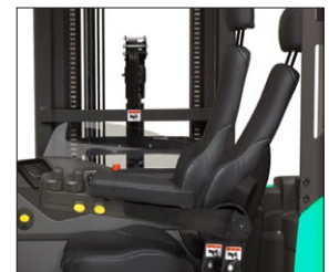
Suspension seat with tilting backrest
